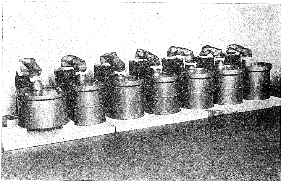
Fig. 1 — Automatic devices for the study of the diurnal activity in insects. The cylindrical vessels with collecting devices are connected by a wire net corridor with isolators from which metamorphosed burying beetles gradually emerge.
